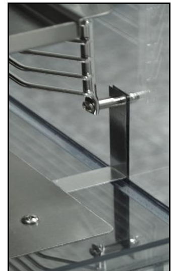
Shield, rack and shelf grounding
